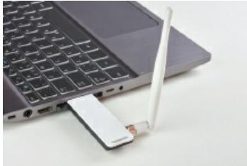
Figure 2.18 Wireless network interface card/controller (WNIC)
