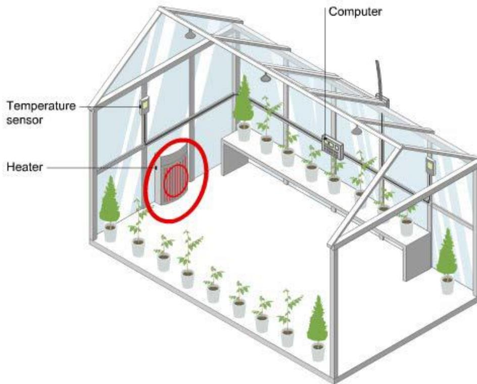
The system monitors the conditions day and night with immediate response to any changes. To alter the growing conditions, the values in the computer program can of course be changed.
